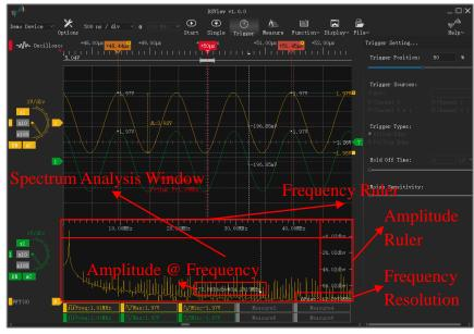
As Figure 3-28 shows, spectrum window display below the wave window.
