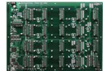
Example of a custom burn-in board
