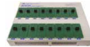
Example of attaching dedicated adapters (TK series)
